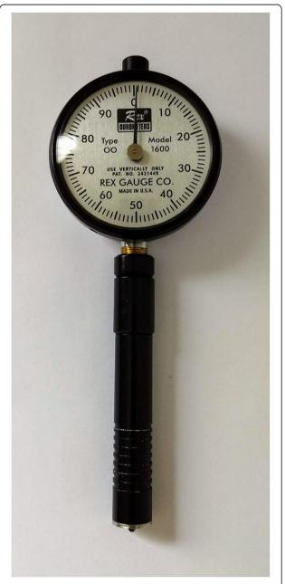
Fig. 1 Durometer model 1600, type 00, Rex Gauge Company, Inc., Buffalo Grove, IL, USA
