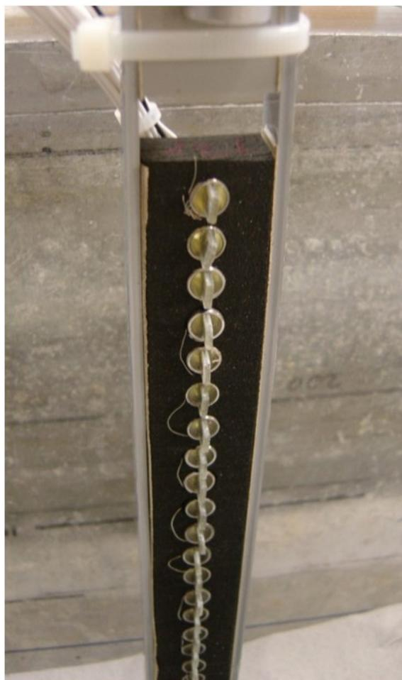
**Figure 5.** Array of bender elements mounted on a tomographic frame.
