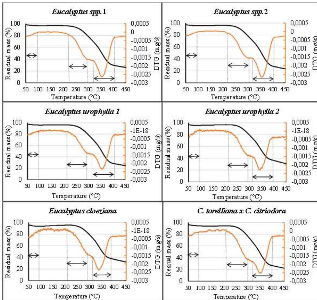
**Figure 1** – Mass loss curves as a function of temperature (TG) and its derivatives (DTG) of the woods of the evaluated clones, with the designation of the ranges with the greatest mass loss.
