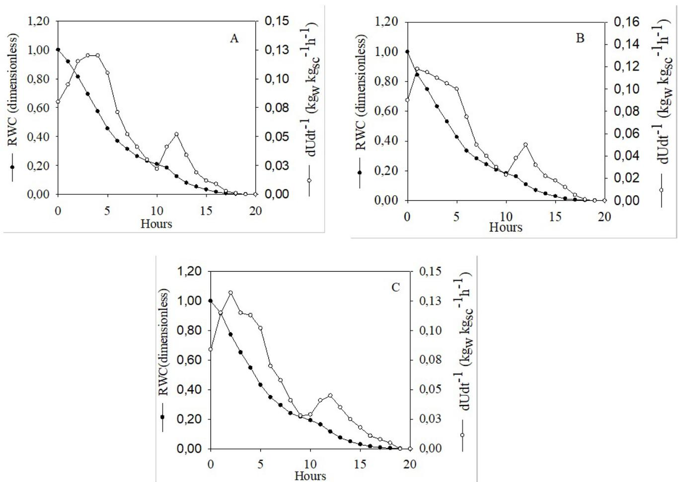
**Figure 3.** Ratio water content (RWC) and drying rate ( $dU/dt$ ) of 'Prata' bananas pretreated in water (a), 1% citric acid (b) and 10% lemon solution (c).
