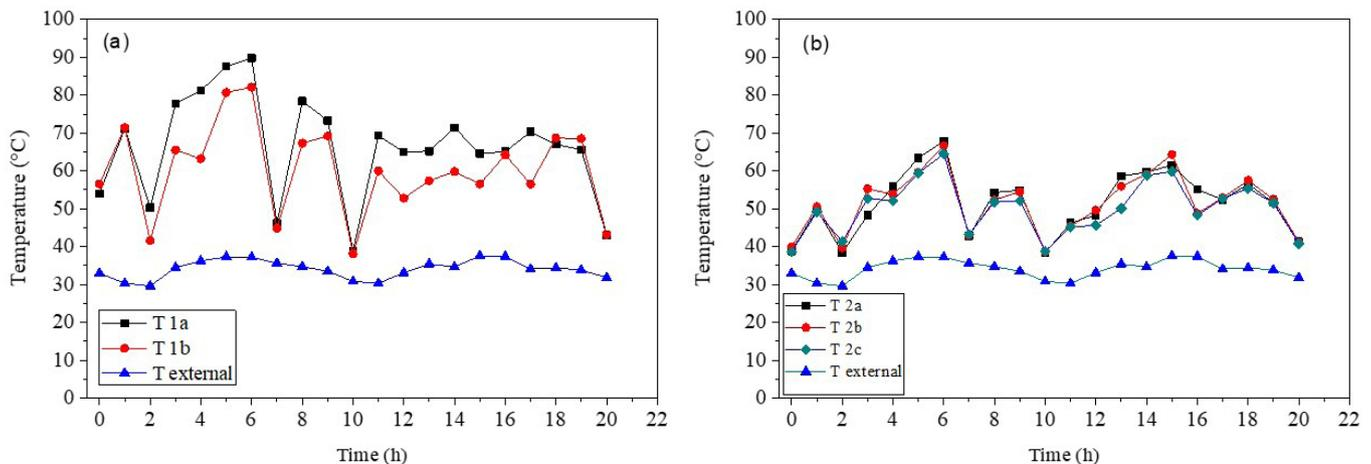
**Figure 2.** Temperature readings in (a) solar collector and (b) drying chamber.
