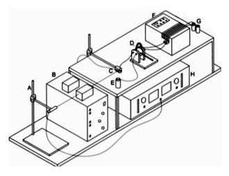
**Figure 1.** FI-SPE-CE system. A: Holder and buffer reservoir; B: Detector; C: Interface; D: injector and column (loop with length 2.5 cm and 0.8 mm of i.d.); E: trash; F: peristaltic pump; G: buffer solution and samples; H: High Voltage source.
