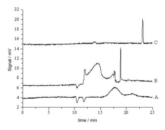
**Figure 2.** FI-SPE-CE electropherograms with pre-concentration of benzoic acid on anionic SPE column. Comparison of 3 eluent solutions. A, sodium hydroxide 1.5 mol  $L^{-1}$ ; B, sodium chloride 1.5 mol  $L^{-1}$  and C, hydrochloric acid 1.5 mol  $L^{-1}$ . Buffer was tetraborate 10 mmol  $L^{-1}$ , pH 10.0, electric field was 250 Vcm<sup>-1</sup>. SPE column with anionic exchange resin Dowex1-X8 (50-100 mesh) was with 2.0 cm long (2 mm i.d.).
