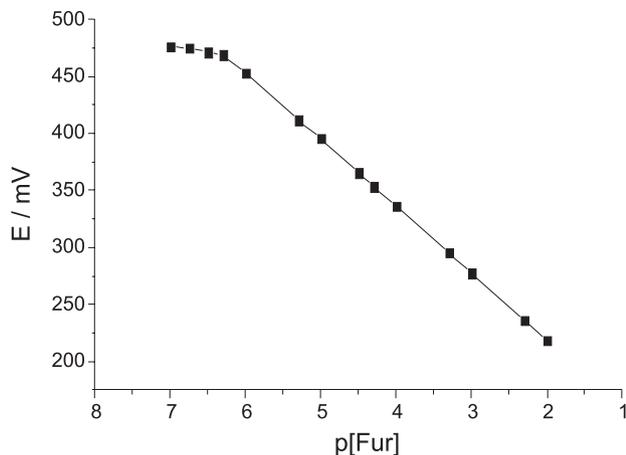
**Figure 2.** Calibration graph for the Fur-sensitive electrode with composition of 50% (Graphite, m/m). Experimental conditions: pH = 8.5,  $\mu = 0.500 \text{ mol L}^{-1}$  adjusted with  $\text{NaNO}_3$ ,  $T = 25 \text{ }^\circ\text{C}$ .
