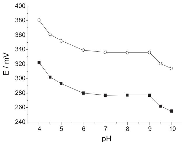
**Figure 3.** Effect of pH on the electrode's response at: (■)  $1.0 \times 10^{-3}$  mol L<sup>-1</sup> Fur, (○)  $1.0 \times 10^{-4}$  mol L<sup>-1</sup> Fur;  $\mu = 0.500$  mol L<sup>-1</sup> adjusted with NaNO<sub>3</sub>, T = 25 °C.
