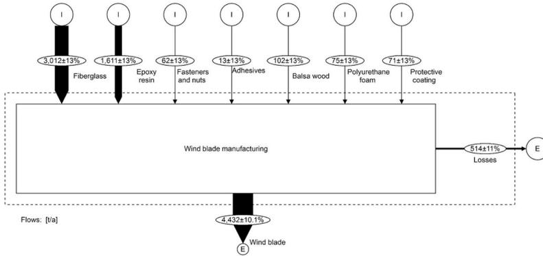
**Figure 2.** Material flow analysis of wind farm blades (onshore model). The flows are classified as import (I) or export (E).
