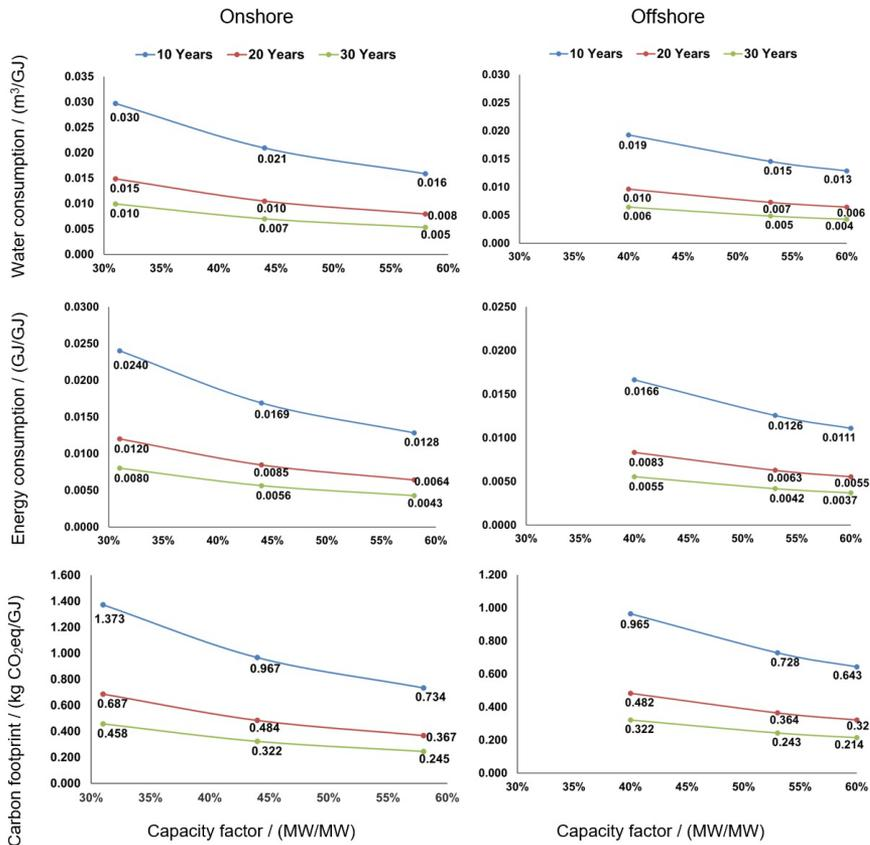
**Figure 5.** Energy and environmental performance of blades for onshore and offshore wind farms per electricity to be produced under different capacity factor and lifetime scenarios.
