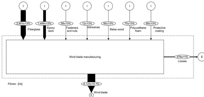
**Figure 3.** Material flow analysis of wind farm blades (offshore model). The flows are classified as import (I) or export (E).
