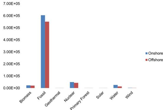
**Figure 4.** Energy consumption of blades for onshore and offshore wind farms by source in GJ.
