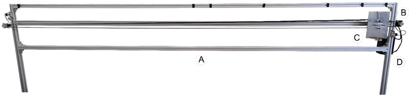
Structure (A), electric drive (B), reading sensor (C), and data acquisition system (D)
