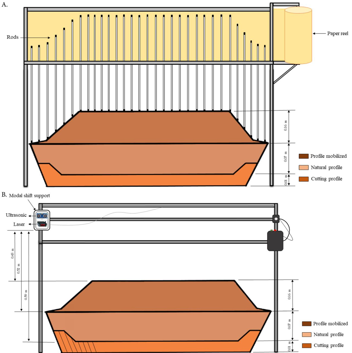
**Figure 3.** Conventional (A) and (B) electronic profilometers were placed laterally to the pot with the mobilized, original/natural, and cut-out soil profiles
