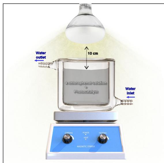
Figure 1. Reactional system used for the photocatalytic tests.
