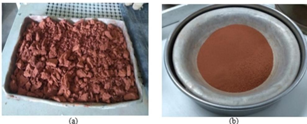
**Figure 1.** (a) Red mud residue before comminution and (b) after hand sieving through a 100 mesh.
