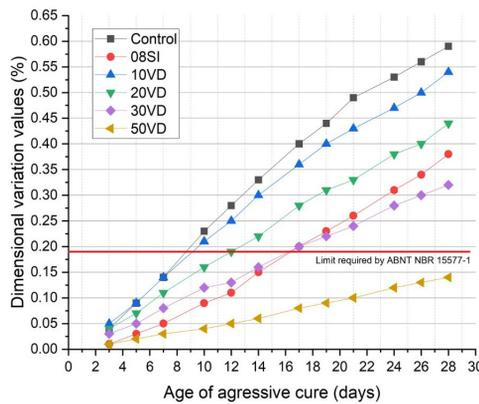
**Figure 5.** Assessment of ASR mitigation with glass powder and silica fume replacing Portland cement.
