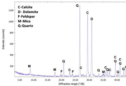
**Figure 3.** Diffractogram of the reactive aggregate.
