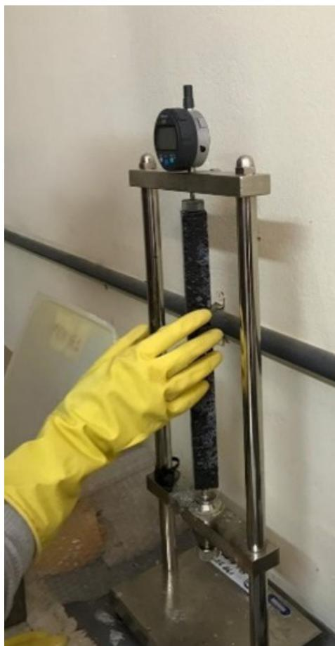
**Figure 4.** Measuring the dimensional variation of the specimens.
