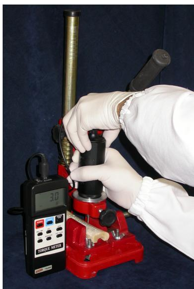
Figure 3. Digital torque gauge (Lutron TQ-8800, Taipei, Taiwan).
