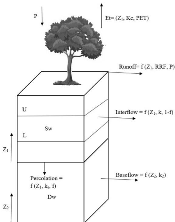
Figure 2. Schematic of the two-layer soil moisture method.
