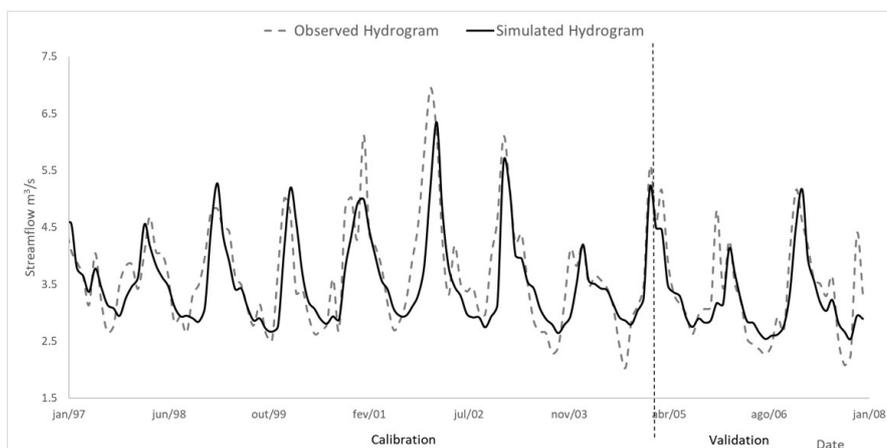
Figure 4. Hydrograph estimated and observed obtained for Feijão Basin (calibration 1997-2004; validation 2005-2007).
