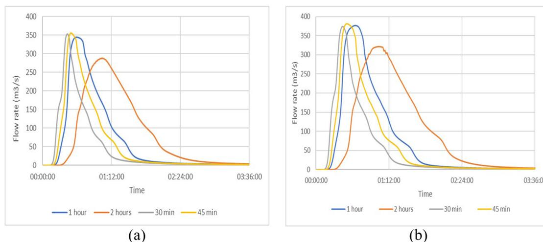
Figure 5. Hydrograms resulting from the design hyetographs with different durations for return periods of 10 (a) and 25 (b) years.
