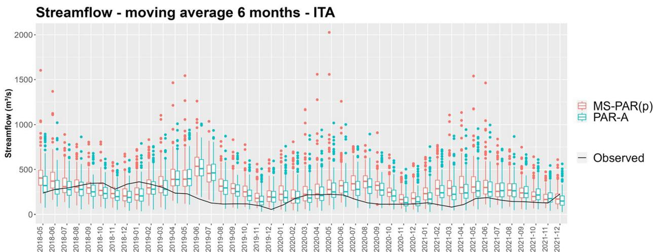
Figure 9. Boxplots of predictive distributions of six-month moving average performed with the MS-PAR(p) (red) and PAR(p)-A (blue), for the Itá HPP.
