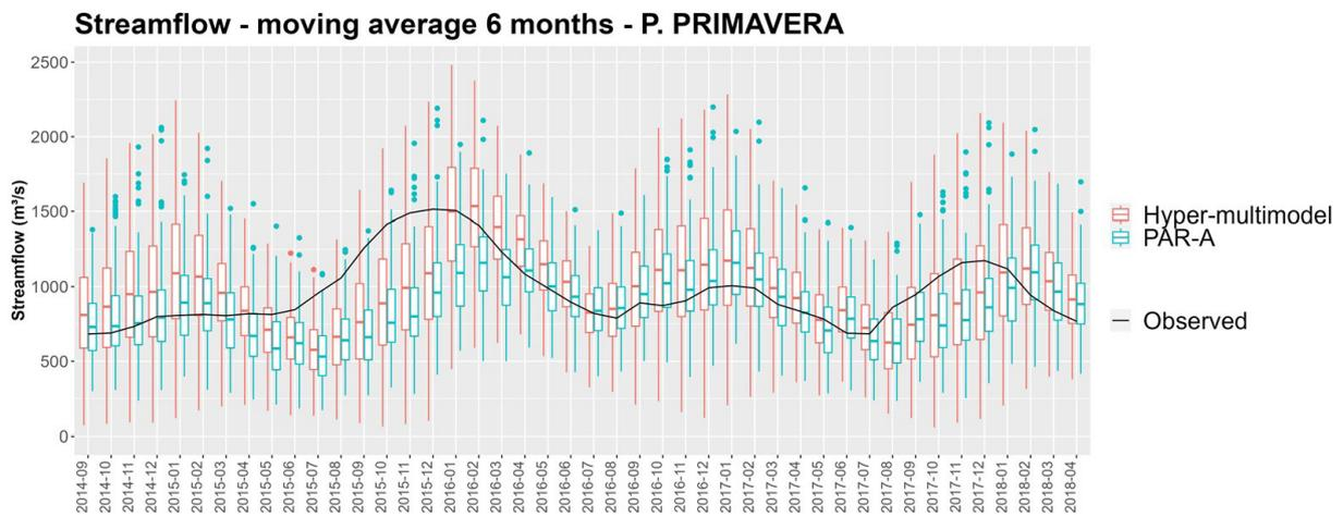
**Figure 14.** Boxplots of predictive distributions of six months moving average performed with the Hyper-multimodel (red) and PAR(p)-A (blue), for the Porto Primavera HPP.
