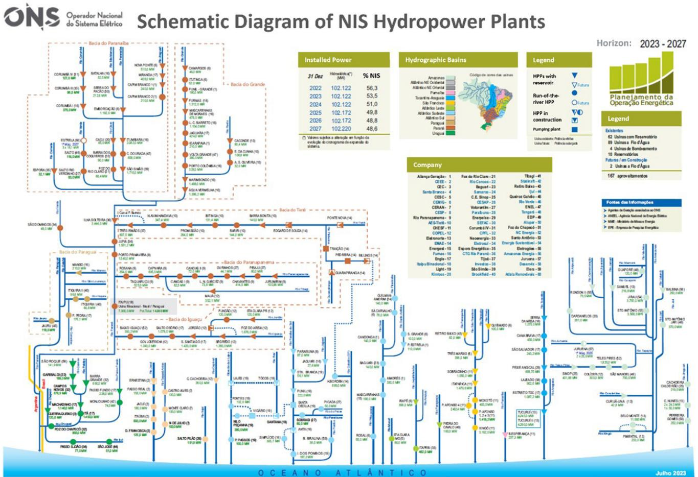
Figure 1. Schematic diagram of the HPPs in NIS.
