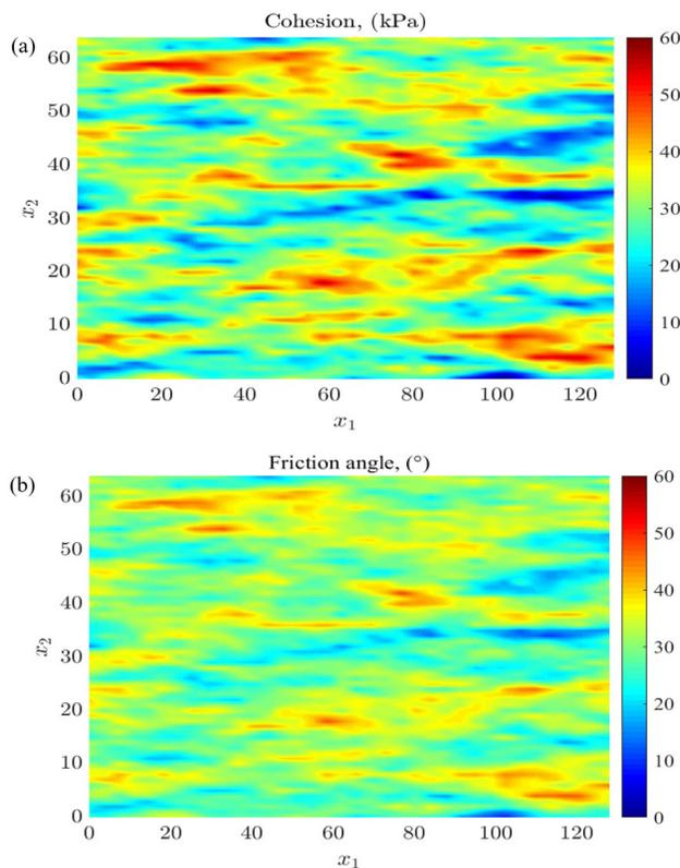
**Figure 2.** Simulation of Gaussian random field with  $\delta_h = 20$  m and  $\delta_v = 2$  m for: (a) soil cohesion with  $\mu_c = 30$  kPa and  $\sigma_c = 9$  kPa; (b) soil friction angle with  $\mu_\phi = 30$  kPa and  $\sigma_\phi = 9$ .
