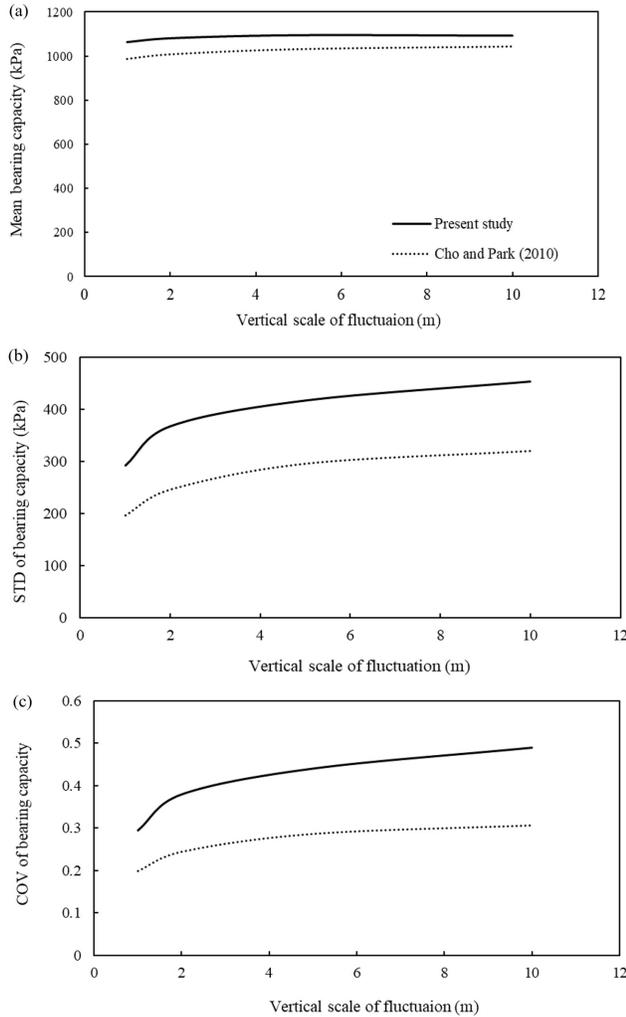
**Figure 6.** Verification of the statistical moment of the bearing capacity of the present study with those of Cho & Park (2010) for a case of  $r(c, \phi) = -0.5$ ,  $COV_c = 30\%$ ,  $COV_\phi = 20\%$ ,  $\delta_h = 10$  m and  $k_h = 0$ : (a) mean, (b) standard deviation and (c) coefficient of variation.
