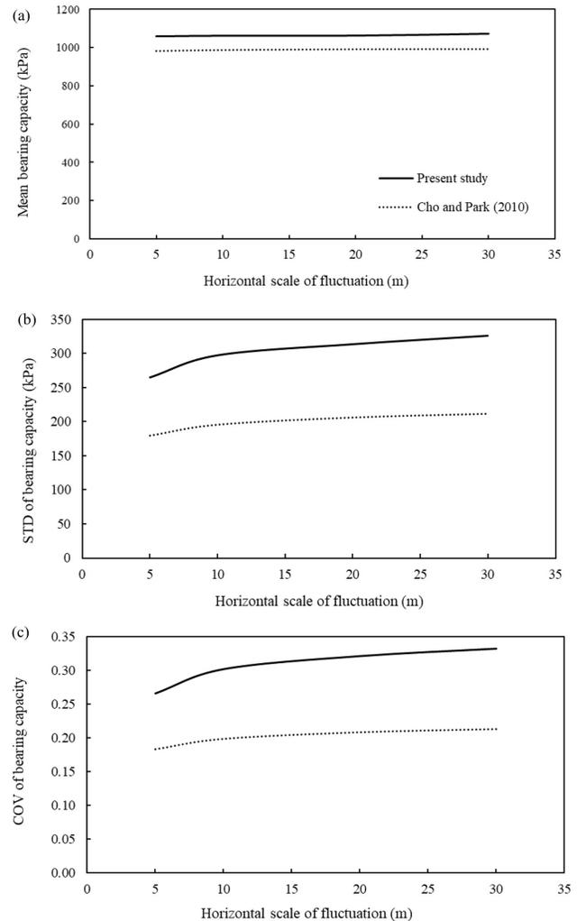
**Figure 5.** Verification of the statistical moments of the static bearing capacity of the present study with those of Cho & Park (2010) for a case of  $r(c, \phi) = -0.5$ ,  $COV_c = 30\%$ ,  $COV_\phi = 20\%$ ,  $\delta_v = 1$  m and  $k_h = 0$ : (a) mean, (b) standard deviation and (c) coefficient of variation.
