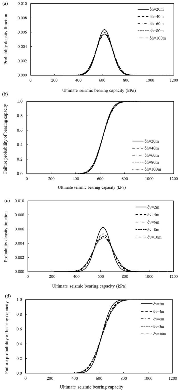
**Figure 11.** Probability density function and failure probability of the seismic bearing capacity of a strip footing resting on cohesive frictional soil for various values of: (a) and (b) horizontal SOF and  $\delta_v = 2$  m, (c) and (d) vertical SOF and  $\delta_h = 20$  m.
