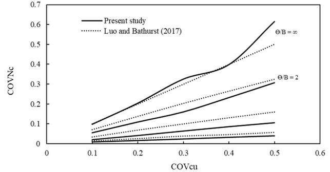
**Figure 4.** Comparison of the  $COV_{N_c}$  of the present study with that of Luo & Bathurst (2017) for a case of  $\mu_{cu} = 20$  kPa,  $\gamma = 20$  kN/m<sup>3</sup> and  $k_h = 0$ .
