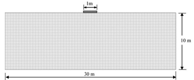
Figure 1. Mesh used for the discretization of random fields.
