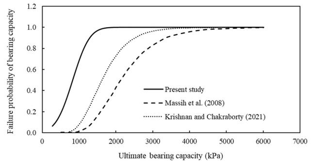
**Figure 7.** Verification of the failure probability of the bearing capacity of the present study with that of Massih et al. (2008) and Krishnan & Chakraborty (2021) for:  $r(c, \phi) = -0.5$ ,  $\mu_\phi = 30^\circ$ ,  $\mu_c = 20$  kPa,  $COV_\phi = 10\%$ ,  $COV_c = 20\%$  and  $k_h = 0$ .
