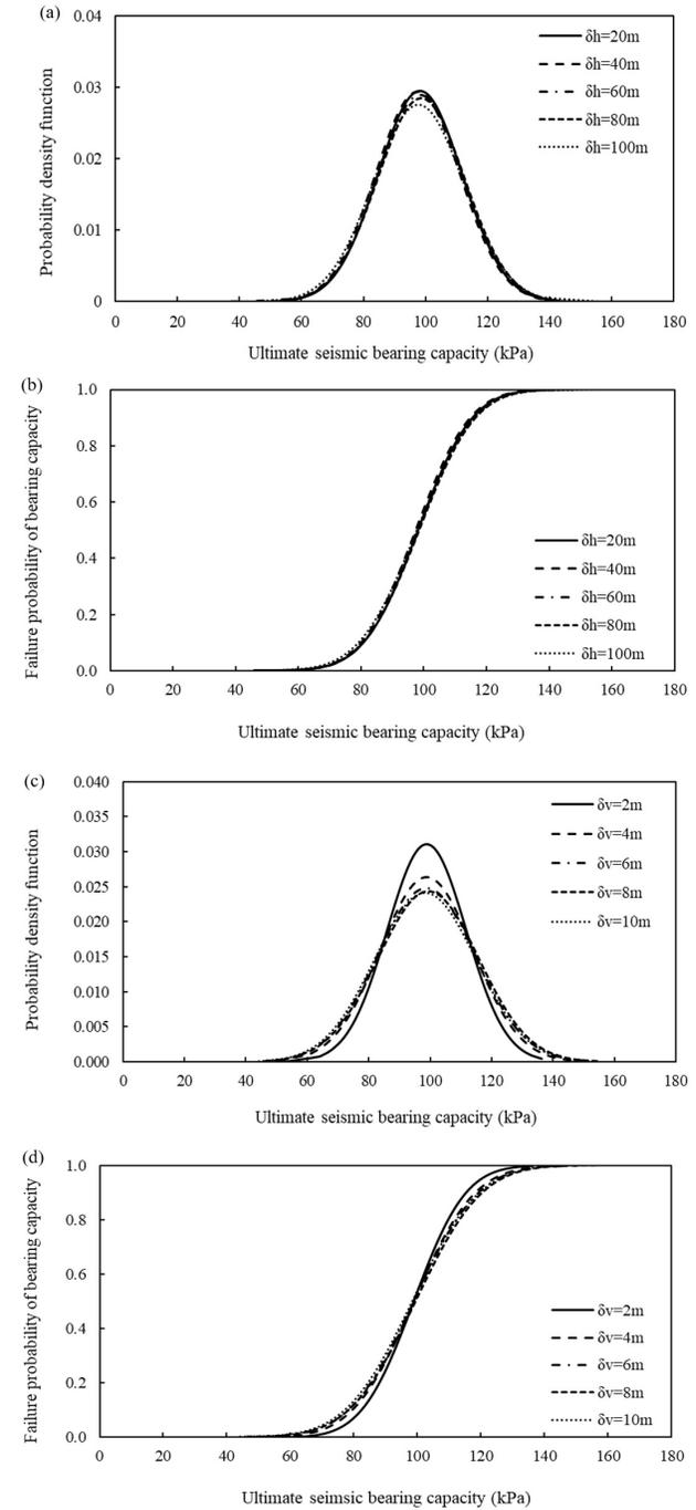
**Figure 12.** Probability density function and failure probability of the undrained seismic bearing capacity of a strip footing resting on a purely cohesive soil for various values of: (a) and (b) horizontal SOF and  $\delta_v = 2$  m, (c) and (d) vertical SOF and  $\delta_h = 20$  m.
