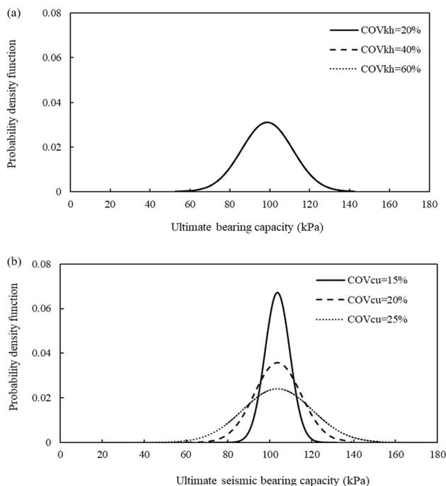
**Figure 10.** The PDF of seismic bearing capacity of strip footing resting on purely cohesive soil for  $\delta_h = 20$  m and  $\delta_v = 2$  m for various  $COV_s$  of: (a) seismic coefficient, (b) undrained shear strength.
