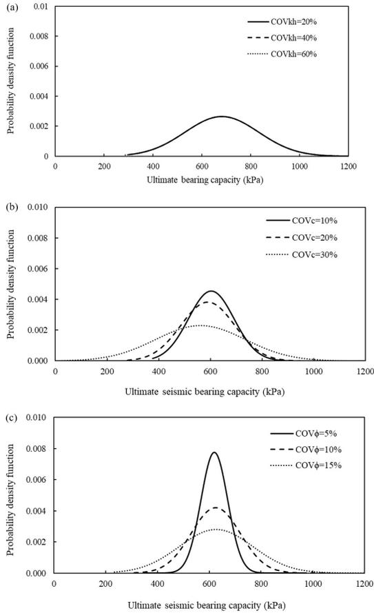
**Figure 9.** The PDF of the seismic bearing capacity of strip footing resting on cohesive frictional soil for  $\delta_h = 20$  m and  $\delta_v = 2$  m for various COVs of: (a) seismic coefficient, (b) cohesion, (c) frictional angle.
