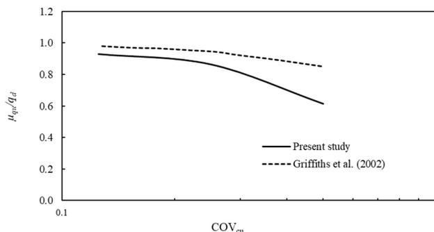
**Figure 3.** Comparison of the normalized bearing capacity of the present study with that of Griffiths et al. (2002) for a case of  $\mu_{cu} = 100$  kPa,  $\delta_x = \delta_y = 2$  m and  $k_h = 0$ .
