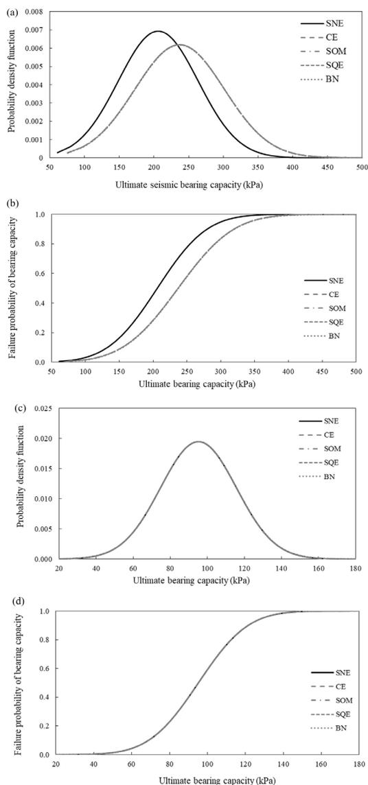
**Figure 8.** Effect of the type of the autocorrelation functions (ACFs), for  $\delta_h = 20$  m and  $\delta_v = 2$  m, on the probability density function (PDF) and the failure probability ( $P_f$ ) of the seismic bearing capacity of a shallow strip footing resting on: (a) and (b) cohesive frictional soil, (c) and (d) purely cohesive soil.
