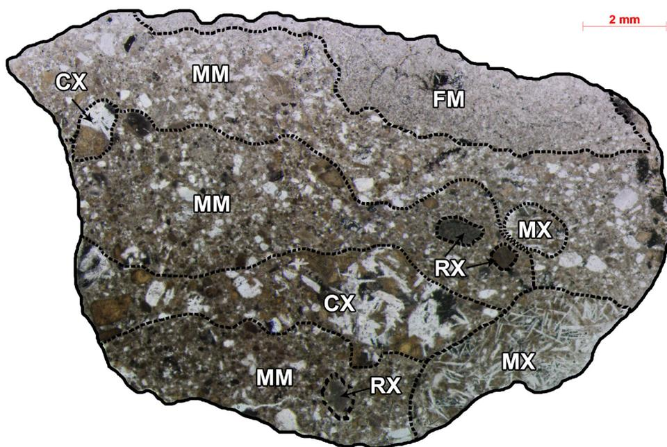
**Figure 2** - Picture of a thin section in transmitted light. A variety of light and dark angular clasts range in size from millimeters to centimeters. The lithologies are outlined with dashed lines for better visualization. The matrix and clasts are identified by letters as indicated in the text of the paper. White areas are plagioclase, medium brown areas are clinopyroxene and small black spots are melts and opaque minerals. The abbreviations are those presented in figure 3.
