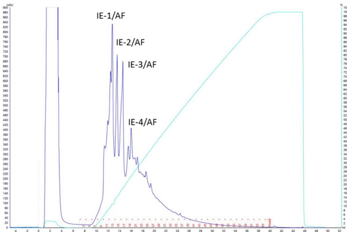
Figure 2. Chromatogram of aqueous fraction (AF) separation using ion-exchange chromatography.
