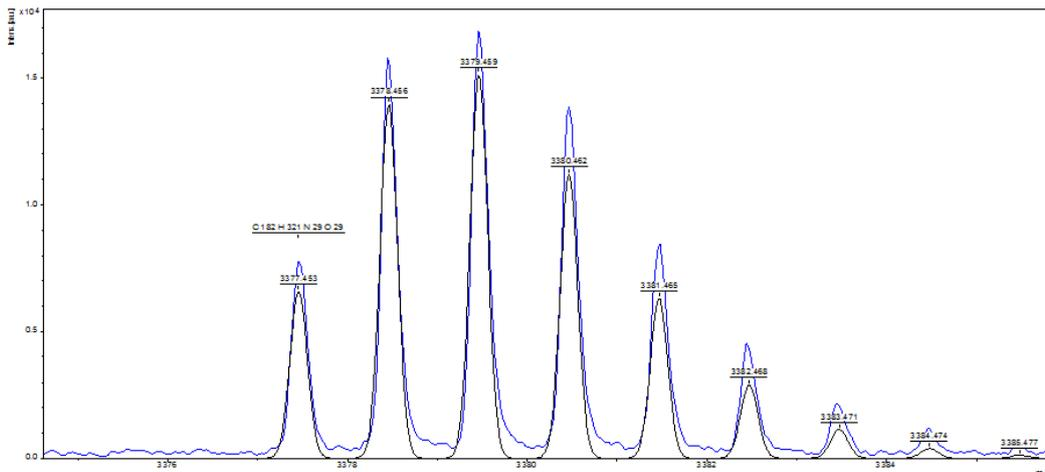
**Figure 7.** MALDI mass spectrum of polycerradin (zoom  $m/z$  3,375 – 3,386). The molecular formula  $C_{182}H_{321}N_{29}O_{29}$  corresponds to a simulation of ion  $m/z$  3,376.459 made by SmartFormula (Flex Analysis software).
