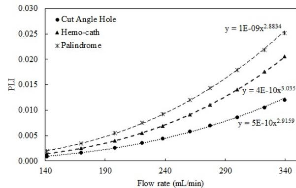
**Figure 3.** Comparison between the PLI values computed at the catheter outlet as a function of catheter flow rate, for each of the CVC analyzed with standard geometry.
