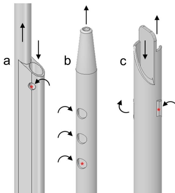
**Figure 1. Representation of the catheter tips used. a) Cut Angle Hole, b) Hemo-cath and c) Palindrome. \*Regions near holes, for shear stress computations.**
