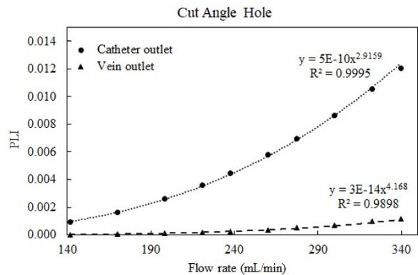
**Figure 2.** PLI variation at the catheter outlet and vein outlet as a function of the flow rate in the CVC (Cut Angle Hole-standard geometry). The arrows indicate the flow direction.
