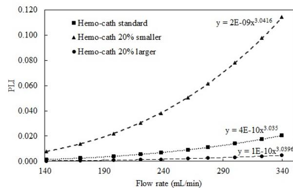
**Figure 4.** Comparison between PLI values computed at the catheter outlet as a function of catheter flow rate, for Hemo-cath with standard geometry, 20% larger and 20% smaller at scale.
