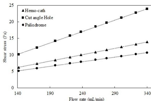
**Figure 5. Variation in the mean value of shear stress as a function of flow rate, in regions near the lateral holes of Hemo-cath, Cut angle hole and Palindrome catheters with the standard size.**
