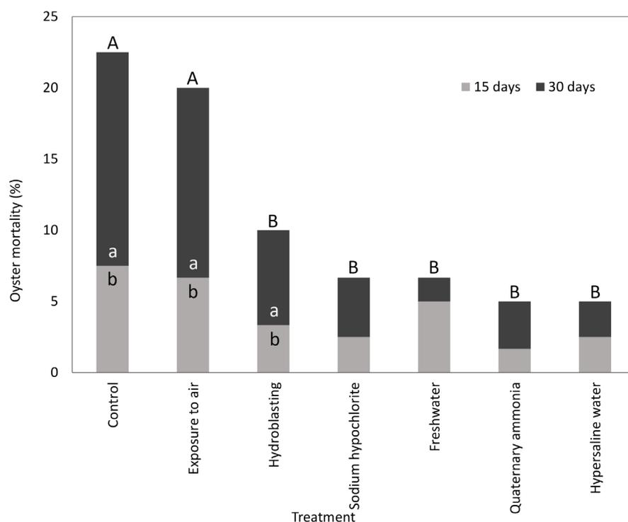
**Figure 4. Cumulative percentage of dead oysters in the control group and in the respective treatments during the experiment for epibiont control. Capital letters indicate differences (Duncan test;  $p < 0.05$ ) among treatments and lowercase letters indicate differences between 15 and 30 days (McNemar Chi-square test;  $p < 0.05$ ).**
