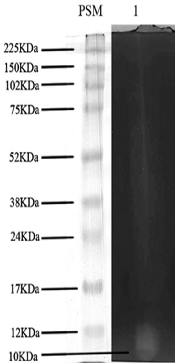
**Figure 3.** Fibrin zymography analysis. Lane PSM, protein size maker by SDS-PAGE analysis; Lane 1, fibrin zymography of the fibrinolytic enzyme purified by ion-exchange chromatography.
