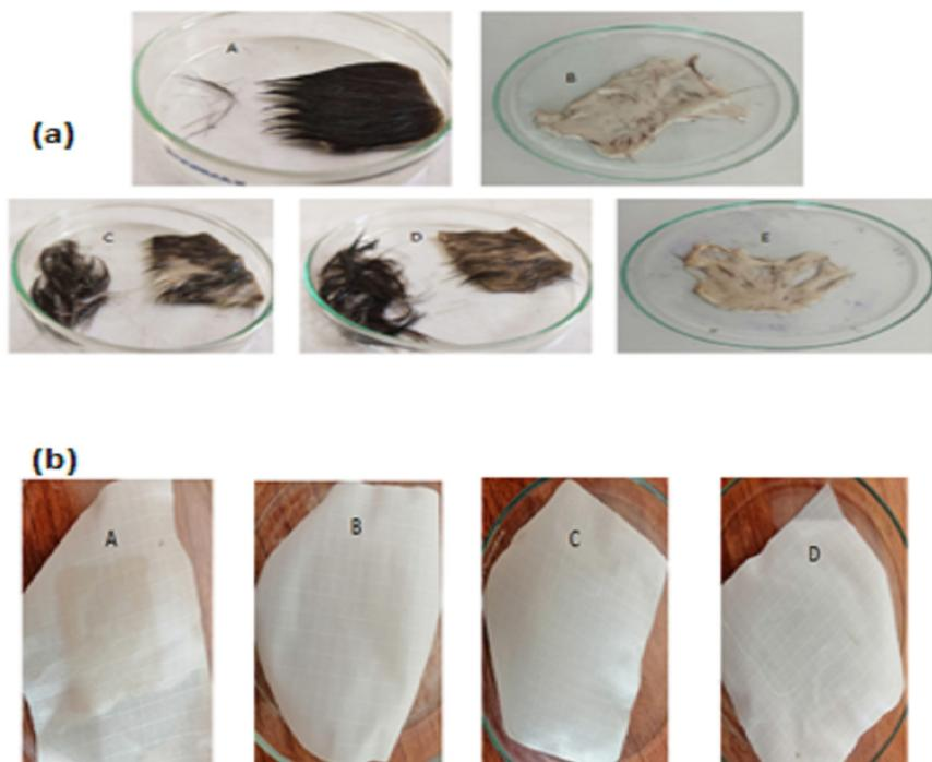
**Figure 6.** (a) Dehairing activity of metalloprotease of TS2; “A” control treated with water only; “B” treated with 10 % lime and 3 % sodium sulfide; “C” treated with 1 % metalloprotease; “D” treated with 2 % metalloprotease and E treated with 3 % metalloprotease; (b) Destaining activity of metalloprotease; “A” control treated with distilled water; “B” treated with commercial detergent; “C” treated with 3 % metalloprotease and “D” treated with detergent plus 3 % protease.
