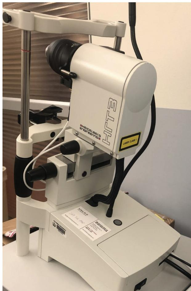
**Figure 1** The HRT3 RCM confocal microscope.
