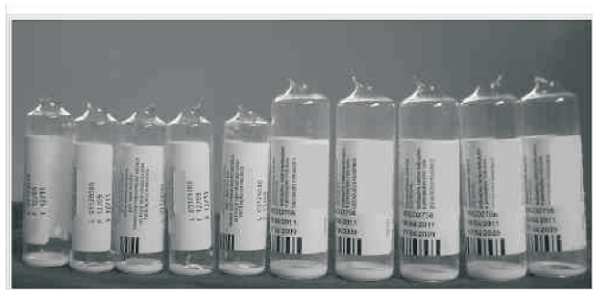
Figure 5 – Vertical Projections on the Opening Border of Propofol Ampoules (10 and 20 mL).
