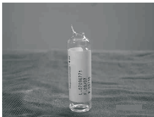
Figure 6 – Vertical Projections on the Opening Border of a 4 mL Ampoule.
