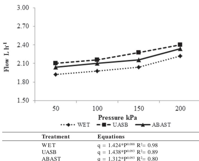
**Figure 2:** Flow curve versus pressure with potential equation for emitters used for subsurface dripping with treated water types and evaluated pressures.
