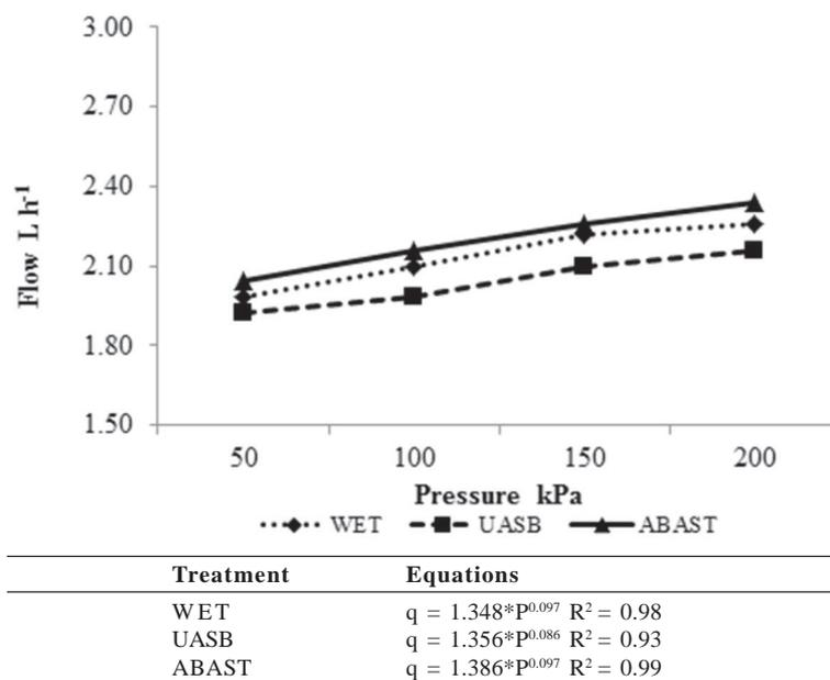
**Figure 1:** Flow curve versus pressure curve with potential equation for emitters used for surface dripping with the types of treated water and evaluated pressures.
