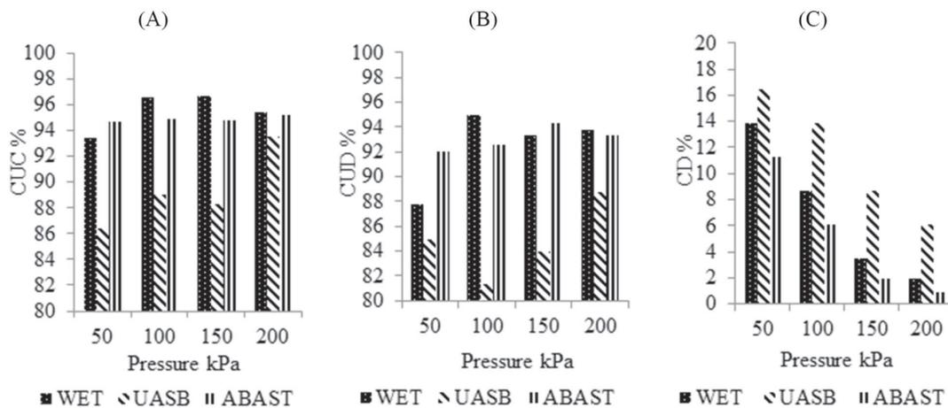
**Figure 3:** Christiansen's coefficient of uniformity (A), coefficient of distribution (B) and clogging degree (C) of emitters used for surface dripping with the types of treated waters and evaluated pressures.
