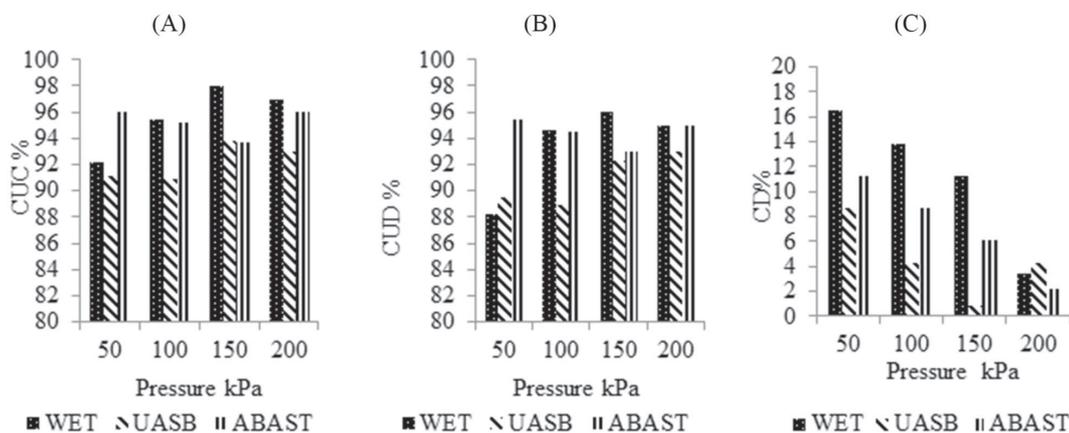
**Figure 4:** Christiansen's coefficient of uniformity (A), coefficient of distribution (B) and degree of clogging (C) of emitters used for subsurface dripping with the types of treated waters and evaluated pressures.
