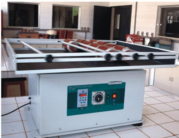
Figure 1. A view of the reciprocal shaker (RSh) as used for the mechanical dispersion of the soil samples using common glass pots.
