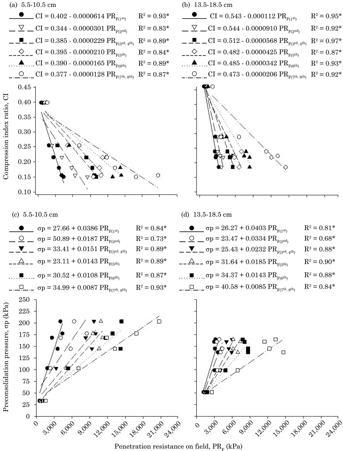
**Figure 6. Correlation between compression index ratio (a, b) and preconsolidation pressure (c, d) with soil penetration resistance, using an impact penetrometer at different water content ranges of a Rhodic Eutrudox in the 5.5-10.5 cm (a, c) and 13.5-18.5 cm (b, d) layers.**
