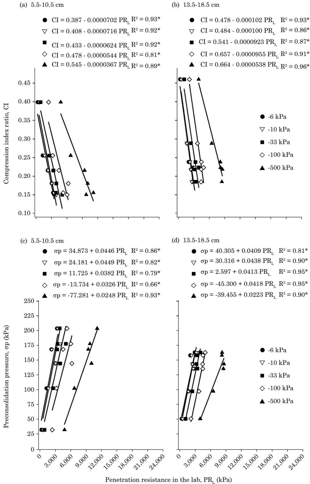
Figure 5. Compression index ratio - CI (a, b) and preconsolidation pressure -  $\sigma_p$  (c, d) with the soil mechanical resistance to penetration of a Rhodic Eutrudox measured with a static penetrometer ( $PR_L$ ) at different soil water potentials, in the 5.5-10.5 and 13.5-18.5 cm layers.
