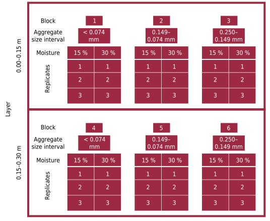
Figure 2. Generalized random block experimental design for soil incubation with two gravimetric moisture levels.
