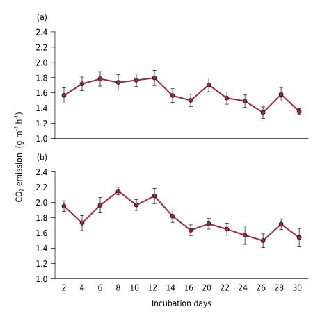
Figure 3. Average  $CO_2$  emission rate under 15 % (a) and 30 % (b) moisture treatments for a calcareous soil in the Comarca Lagunera, Mexico.
