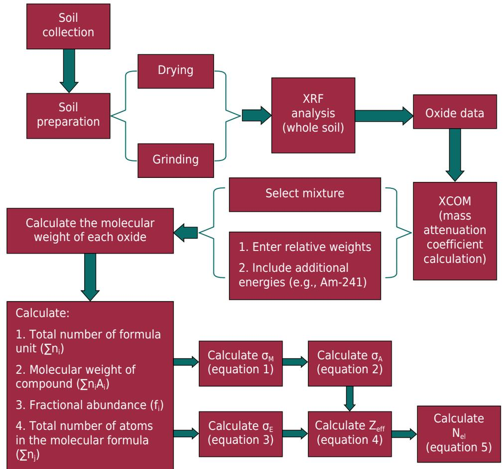
**Figure 2.** Flowchart of the procedures utilized for calculating the soil radiation interaction parameters.
