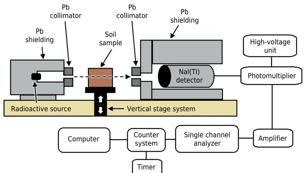
**Figure 3.** Scheme of the gamma-ray attenuation system.
