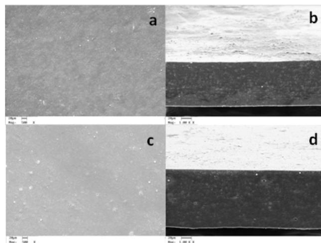
**Figure 6.** Scanning electron microscopy of canihua flour films. **a.** Surface of the film FCC, **b.** Cross-sections of the film FCC, **c.** Surface of the film FCII **d.** Cross-sections of the film FCII
