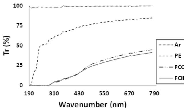
**Figure 3.** Light transmittance (Tr) of canihua films of the varieties (FCC) *cupi* and (FCII) *illpa-inia* and light transmittance of air (Ar) as compared with light transmission of a polyethylene film (PE)
