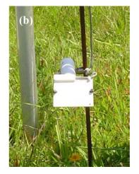
FIGURE 3. Wetness sensors inside the vineyard (a) and at the standard weather station (b), in Jundiaí - SP, Brazil.
