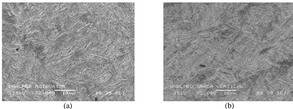
FIGURE 4. Typical aspect of the microstructure of the tools. a) AISI 15B30 steel used in rotary tiller and small motorized rotary tiller, b) AISI 1010 steel used in rotary power harrow. In all cases the structure is composed of tempered martensite.
