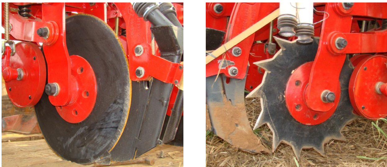
FIGURE 3. Aspect of the cultivator with a chiseling shank, smooth disk (left), and toothed disk (right).
