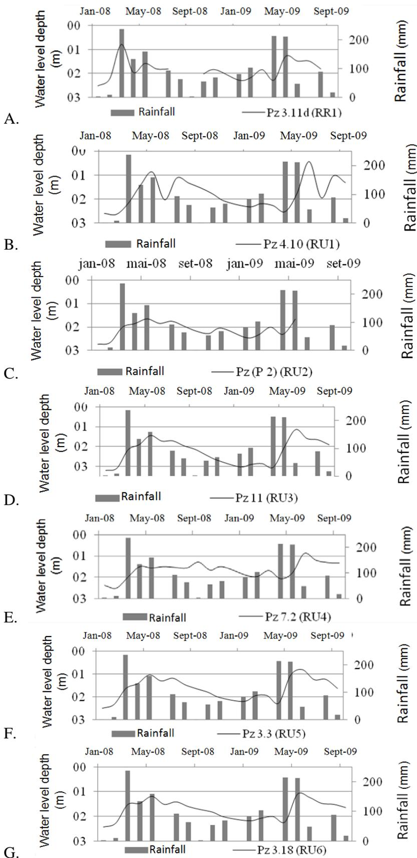
FIGURE 4. Temporal variation of precipitation and the aquifer potentiometric levels. (A) RR1 Entisol + Udorthent; (B) RU1 Entisol; (C) RU2 Fluvent; (D) RU3 Fluvent; (E) RU4 Fluvent; (F) RU5 Fluvent; (G) RU6 Fluvent.
