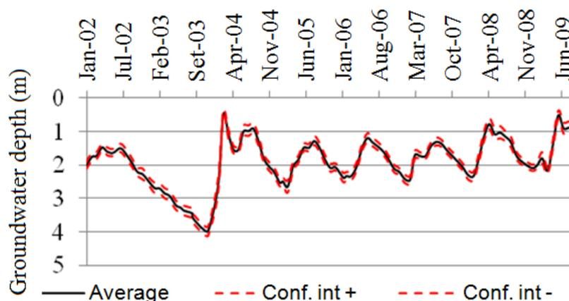
FIGURE 3. Confidence interval for the average piezometric fluctuations. (A) loam soil; (B) sandy loam soil.
