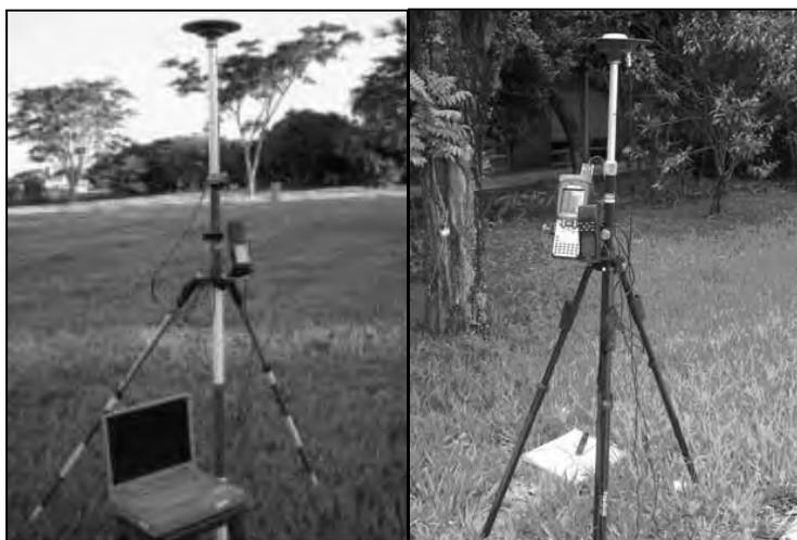
FIGURA 1. Sistema GPS de baixo custo: a) com notebook, e b) com coletora (Fonte: MIYASHITA, 2008). **GPS system for low cost: a) with notebook, and b) with collector (Source: MIYASHITA, 2008).**
