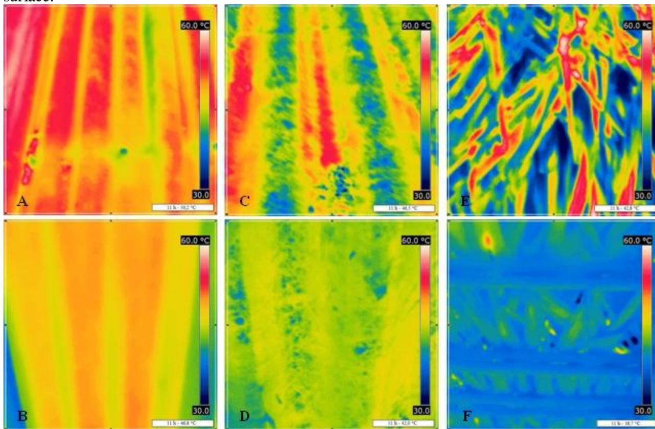
FIGURE 2. Thermographic images from upper and lower surfaces of different roofing materials: fibre cement tile – upper (A) and lower (B); recycled tile - upper (C) and lower (D); thatched roof - upper (E) and lower (F). These images were taken on February 24, 2012, at 11 am, being captured at a distance of 0.50 m.
