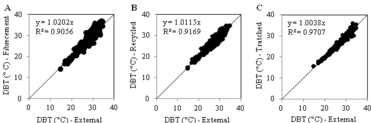
FIGURE 1. Functional relationships between external (environment) and internal temperatures of shelters covered with fibre cement tile (A), recycled tile (B) and thatched roof (C). DBT - dry bulb temperature.
