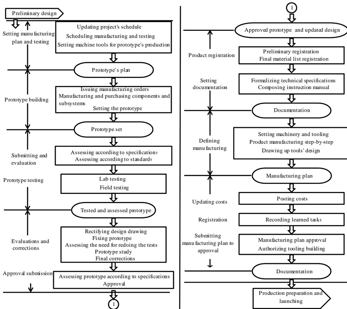
FIGURE 5. Scheme of the detailed design phase.
