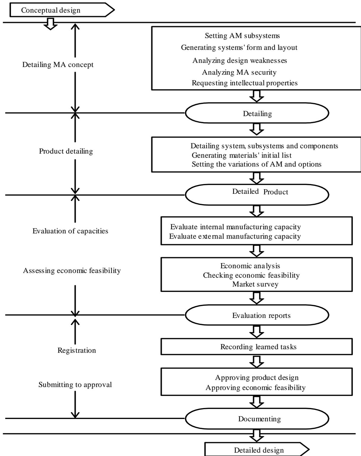
FIGURE 4. Scheme of the preliminary design phase.
