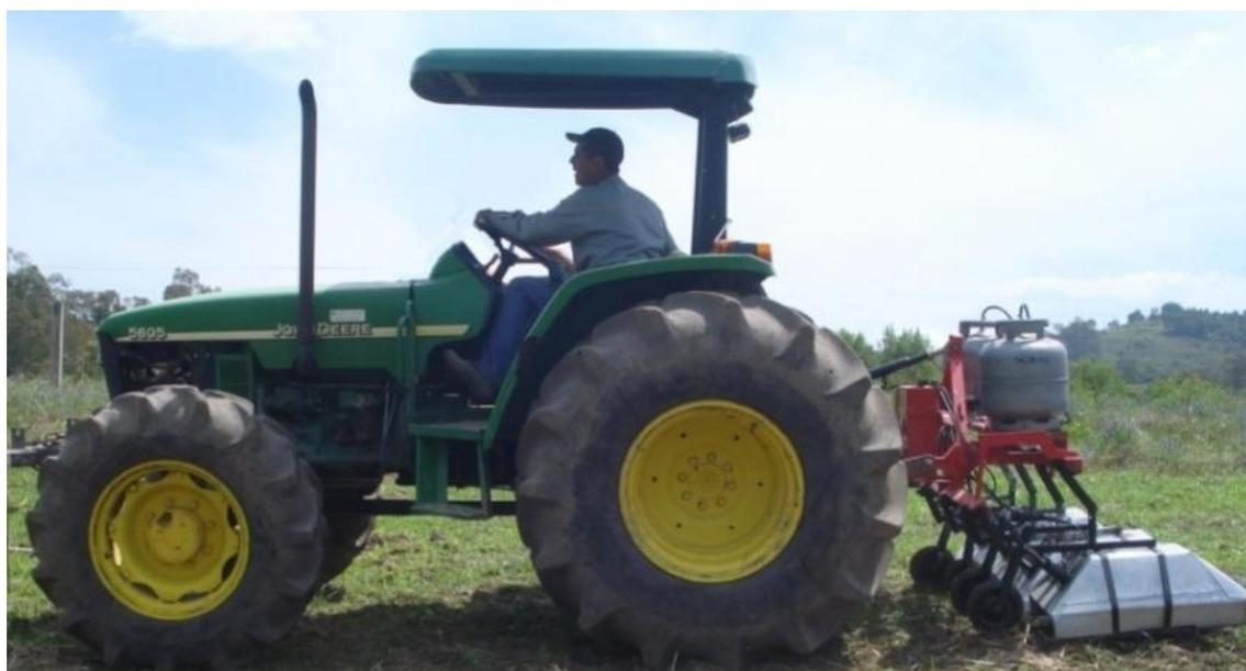
FIGURE 1. Tractor and heat-applicator machine assembly.
