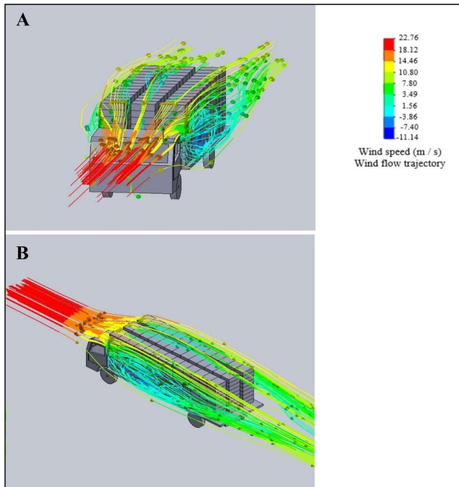
FIGURE 4. Ventilation pattern in the air aisle layout used for transporting live broiler: front (A) and side (B) views of the truck.
