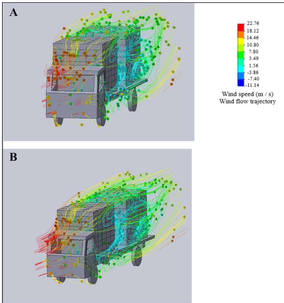
FIGURE 5. Ventilation pattern in the “central span” layout used for the transport of live broiler: front (A) and side (B) views of the truck.
