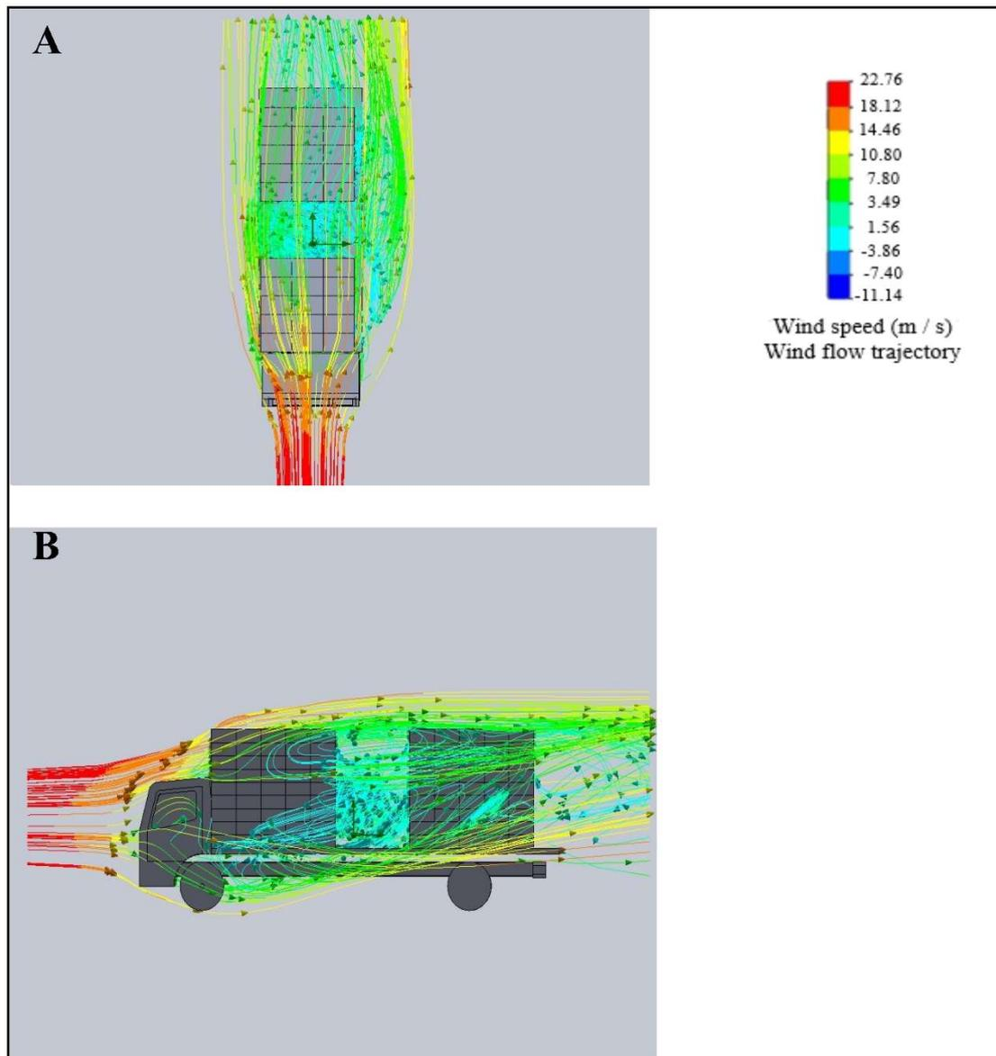
FIGURE 6. Ventilation pattern in the air aisle layout used for transporting live broiler: top (A) and side (B) views of the truck.
