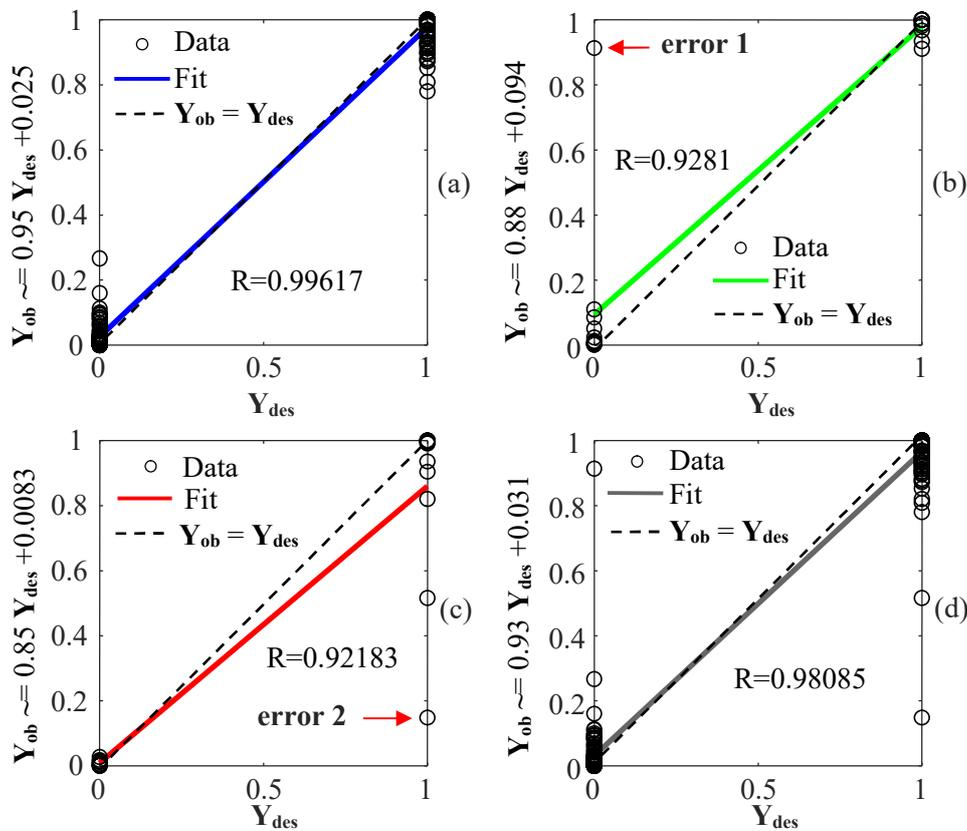
FIGURE 3. Regression analysis between variables: desired output ( $Y_{des}$ ) and obtained output ( $Y_{ob}$ ), (a) training with 80% of the samples, (b) validation with 10% of the samples, (c) test with 10% of the samples and (d) all samples (100%).
