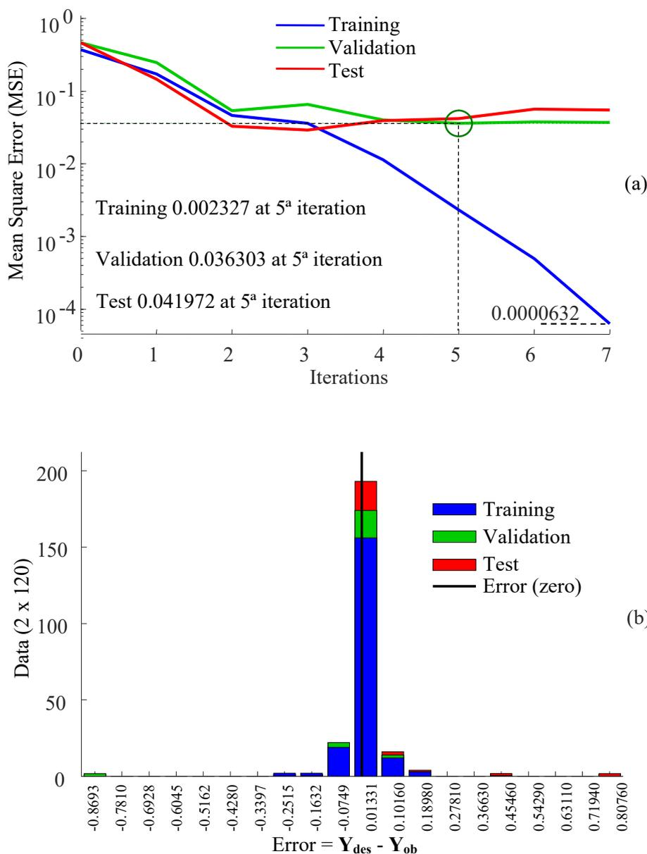
FIGURE 2. Training, validation and test of the ANN, (a) performance (MSE), (b) error histogram ( $Y_{des} - Y_{ob}$ ) with 20 intervals for the 120 output samples (2 x 120 data).
