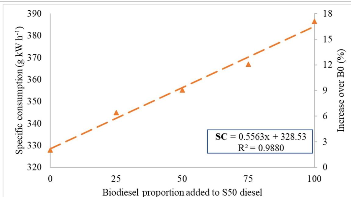
FIGURE 3. Specific fuel consumption as a function of the proportion factor.
