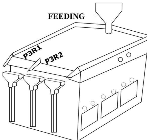
FIGURE 2. Densimetric table set to the seed reprocessing.
