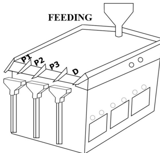
FIGURE 1. Densimetric table set to the seed processing.
