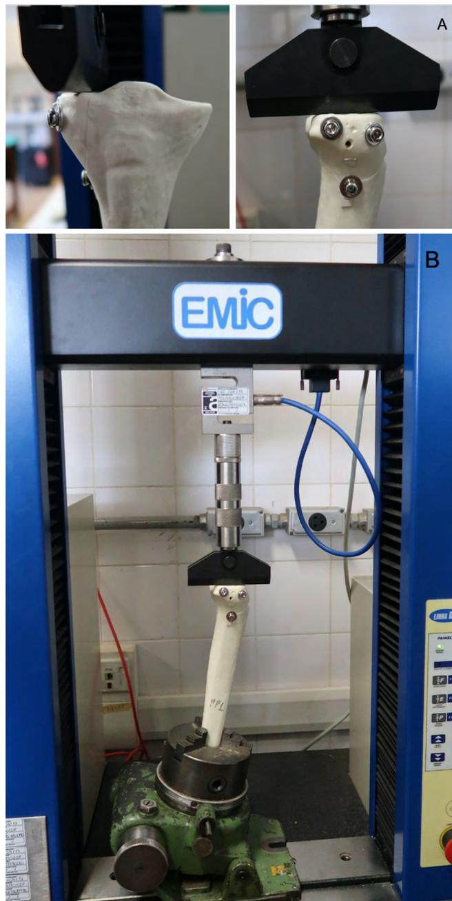
**Figure 3.** – A, Frontal and lateral view of the loading device with a screw-washer construction group model before testing; B, Universal testing machine setup for biomechanical testing.
