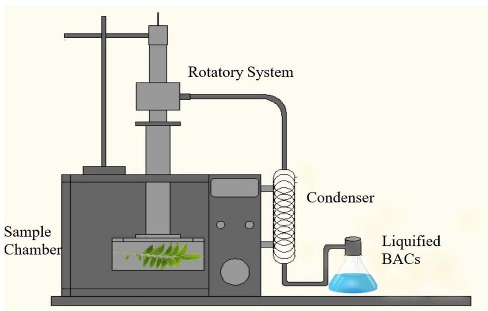
**Figure 1.** Experimental setup for Microwave based drying of fenugreek leaves.
