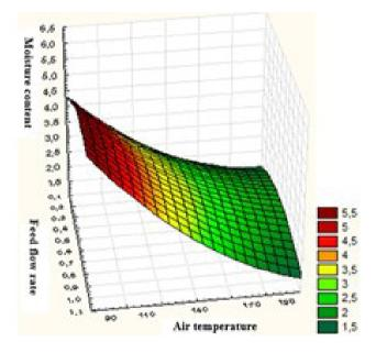
**Figure 3**. Response surface of moisture content of atomized yellow mombin particles as a function of feed flow rate (0.20 to 1.00 L/h) and air temperature.
