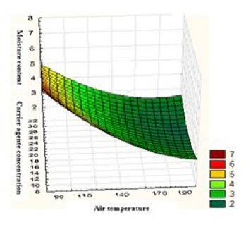
**Figure 2**. Response surface of moisture content of atomized yellow mombin particles as a function of carrier agent concentration (10 to 30%) and air temperature.
