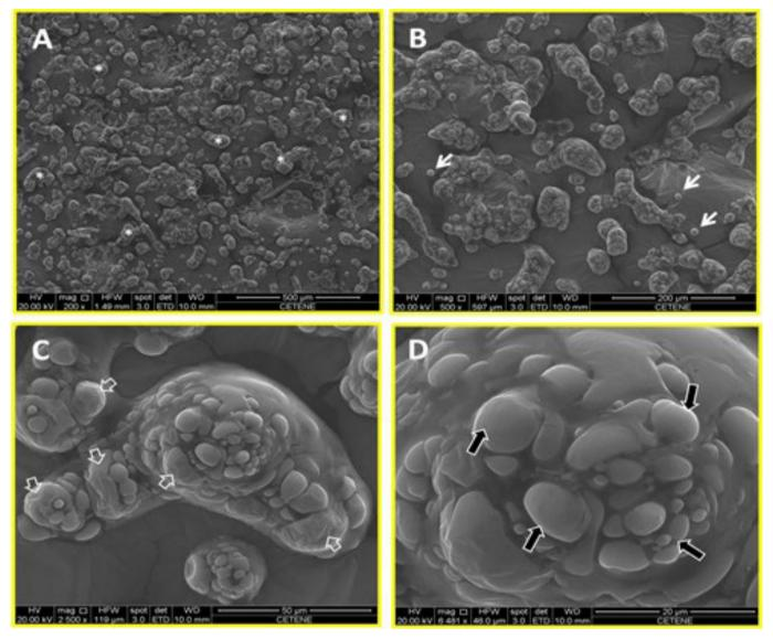
**Figure 4**. (A-D): Electromicrographs of atomized yellow mombin particles. A – Overview of the distribution of particles in the form of agglomerates with different size (asterisks); B – Isolated particles (short arrows); C and D – Details of the agglomerate formed by particles of different size that had a rough surface (open arrow) and a smooth surface (closed arrow).
