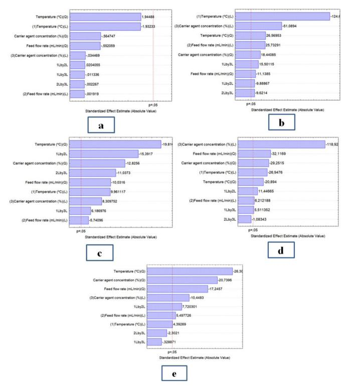
Figure 1. Pareto charts of dependent variables: (a) water activity, (b) moisture, (c) hygroscopicity, (d) process yield, and (e) total carotenoids retention.
