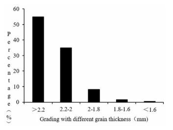
Figure 1. Grading of average grain thickness.
