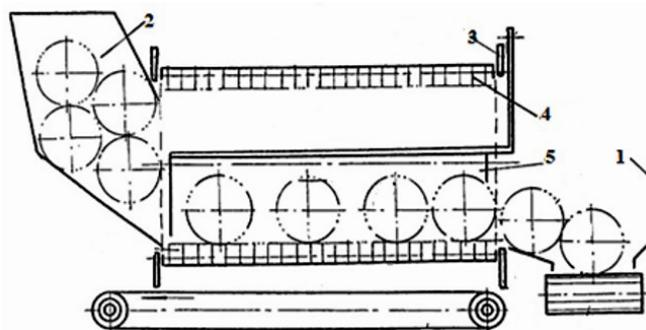
**Figure 1.** Arrangement of equipment for cleaning cucurbit crops: 1 – frame, 2 – hopper, 3 – drum, 4 – brushes, 5 – additional brush.
