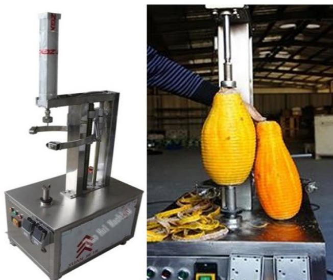
Figure 4. Watermelon peeling machine (China).
