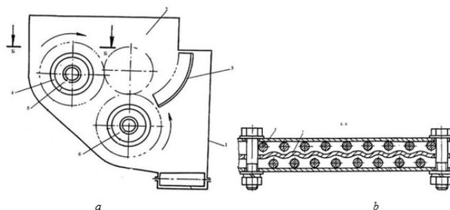
**Figure 2.** Arrangement of equipment for cleaning cucurbit crops: a – vertical section of the equipment; b: 1 – frame, 2 – hopper, 3 – retaining brush, 4 – hollow roll, 5,6 – drums, 7,8 – rope.
