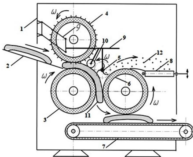
**Figure 3.** Equipment for cleaning cucurbit crops: 1 – frame, 2 – tray, 3 – support roll, 4 – needle roller, 5 – milling drum, 6 – clamping roll, 7 – conveyor of peeled slices, 8 – peel conveyor, 9 – holder, 10 – copying wheel, 11 – fruits, 12 – peel.
