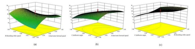
Figure 5. Influence of interactive factors on the splitting into two flaps. (a) Interaction between harvester forward speed and threshing roller speed; (b) Interaction between harvester forward speed and deflector angle; (c) Interaction between the threshing roller speed and deflector angle.
