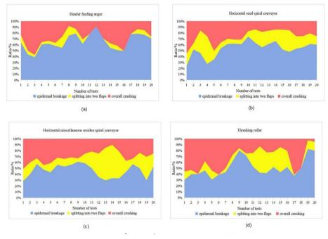
**Figure 3**. Distribution of different crushing forms in main operation process. (a) Header feeding auger; (b) Horizontal seed spiral conveyor; (c) Horizontal miscellaneous residue spiral conveyor; (d) Threshing roller.
