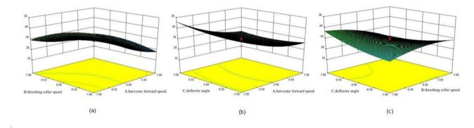
**Figure 6**. Influence of interactive factors on the overall crushing. (a) Interaction between harvester forward speed threshing roller and threshing roller speed; (b) Interaction between harvester forward speed and deflector angle; (c) Interaction between the speed and deflector angle.
