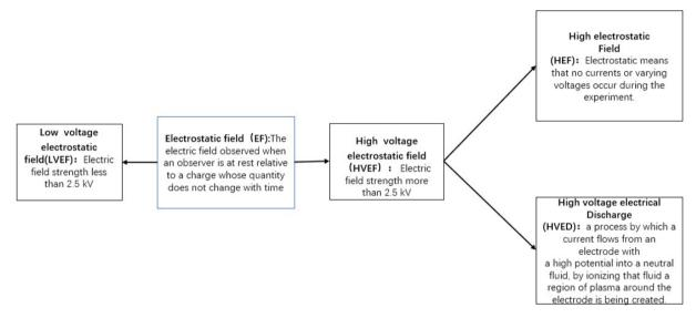
Figure 7. Characteristics of different EF plant.
