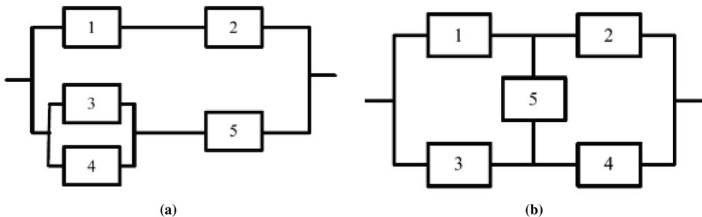
**Figure 2** – Configurations of the systems for Problems 1 (a) and 2 (b).
